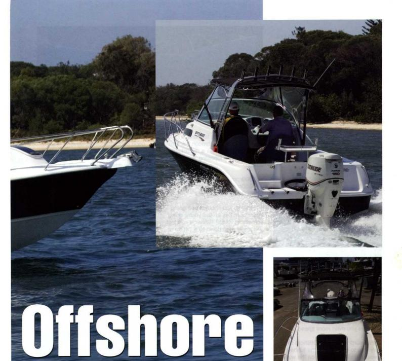
However, what really excites even more about the 595 Offshore is the revolutionary 'tunnel' bottom shape we first saw in the Freedom 640 Seasport two years ago. Starting with a deep Vee hull of approximately 21-degrees deadrise the Freedom features the clever addition of a hollow tunnel down the keel centre line that tapers out up near the forefoot.
