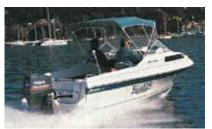
The Freedom displayed a reasonably good ride in broken water, though at times landed hard due to the wide side chines.
