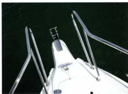
Split rail makes bow access easy.
